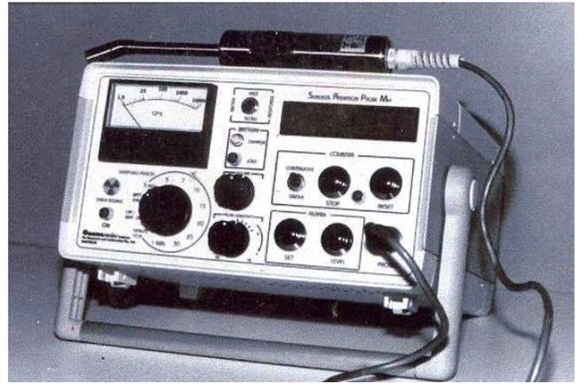
Figure 1. Gamma ray detecting probe.
