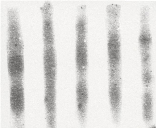
Figure-3: The radiographic image of the phantom sheet. The density difference between the strips and the sheet was similar to that between bone and muscle tissues.
